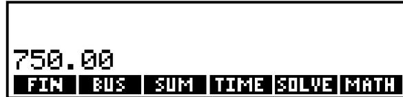
The *first operand* of the initial calculation is *displayed*, but the number stored in Rn, 9000, is correct. Neither DISP nor PRNT redress the display; to do so just press RCL n:
