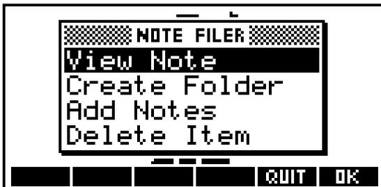
A 39G screen captured by pressing ON-PLOT and then executing PRVAR G0. On the 38G and 39G, ON-1 always dumps to the serial port.
